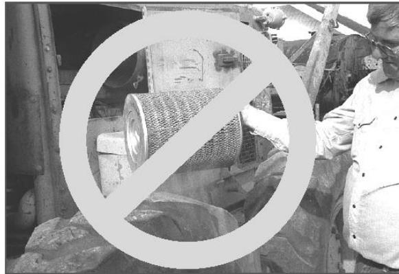
Do **NOT** bang the air filter against a tire or other object. Doing so will distort the shape of the filter, degrading the seal to the intake. If the filter is dirty, replace it!
