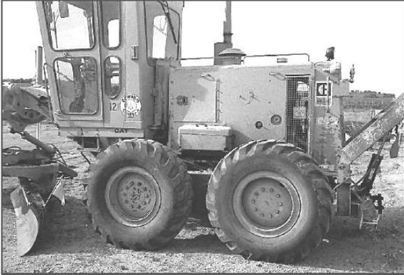
Mismatched tires cause internal wear on the drive chains and differential. Using mismatched tires does **not** save money.
