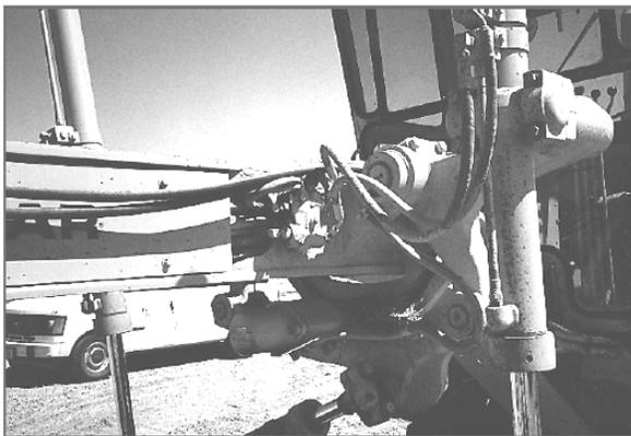
Loose hoses are a breakdown waiting to happen. Hydraulic hoses that have been added to the machine must be of the proper pressure rating and secured to the frame with clamps or brackets.
