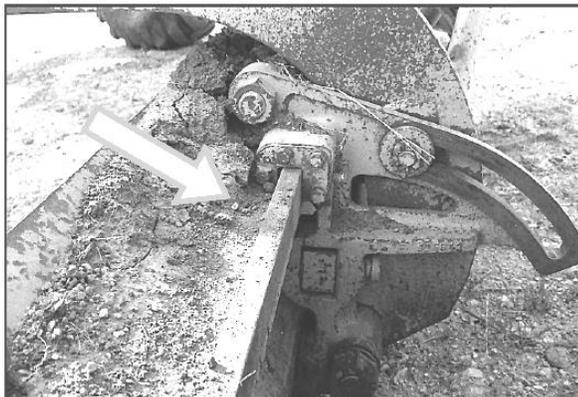
Accumulated debris will cause excessive wear on the shims. Keep the blade slide area clean.
