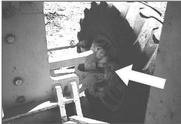
Check the spindles for excessive wear and play.
