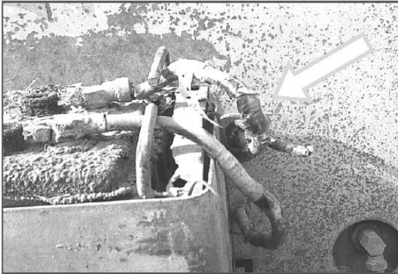
Battery cables that are in poor condition cannot carry the current needed to start the engine and are an electrical hazard. Replace immediately.
