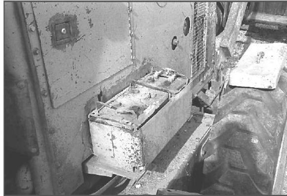
Keep the top of the batteries clean. Accumulated dirt attracts moisture, and this mixture can drain the battery's charge.
