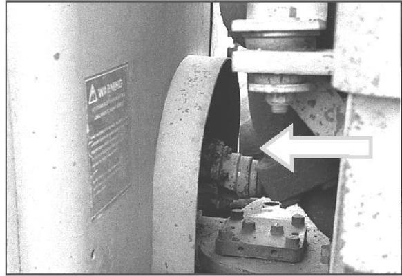
Be sure to replace the safety guard if you remove it to grease the drive shaft. The guard is there to protect you and your co-workers from injury.
