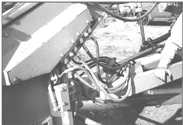
Hoses that have been replaced must be the proper length and secured in the same way as the originals.
