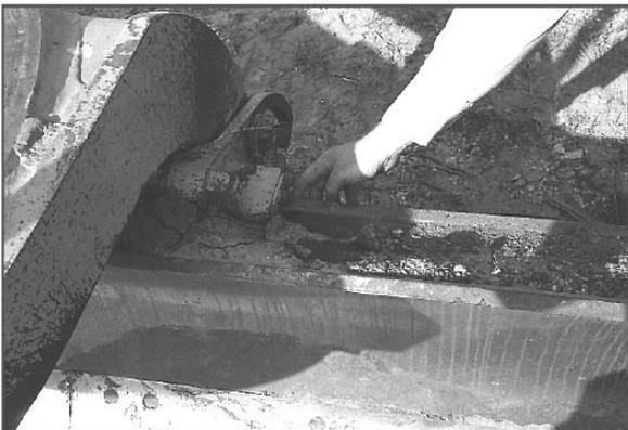
Check the condition of the blade slide. Keep the shims adjusted according to the manufacturer's specifications.
