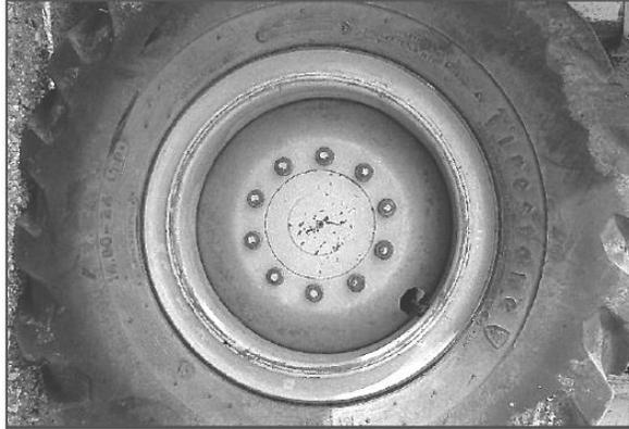
Check all lug nuts. Because of the vibration experienced during grading operations, lug nuts can become loose.
