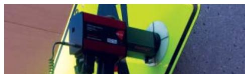
A retroreflectometer provides agencies the means to accurately and consistently assess the condition of signs; it removes the subjectivity of visual sign inspection. A major drawback to using a retroreflectometer is the high initial investment. The purchase price of a new one is \$8,000 to \$15,000, depending on optional features.
