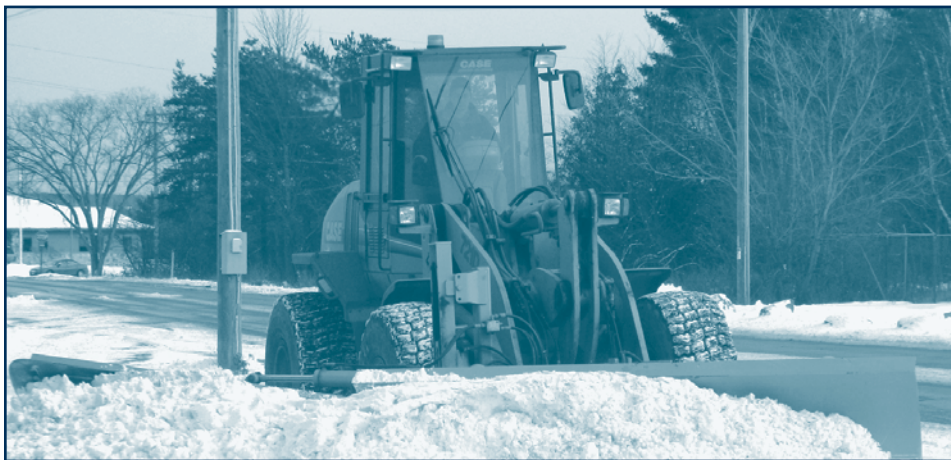
Mark Zenner, director of DPW for the City of Houghton, demonstrates how a wheeled loader-mounted plow clears a 22 foot wide path in a single pass.
