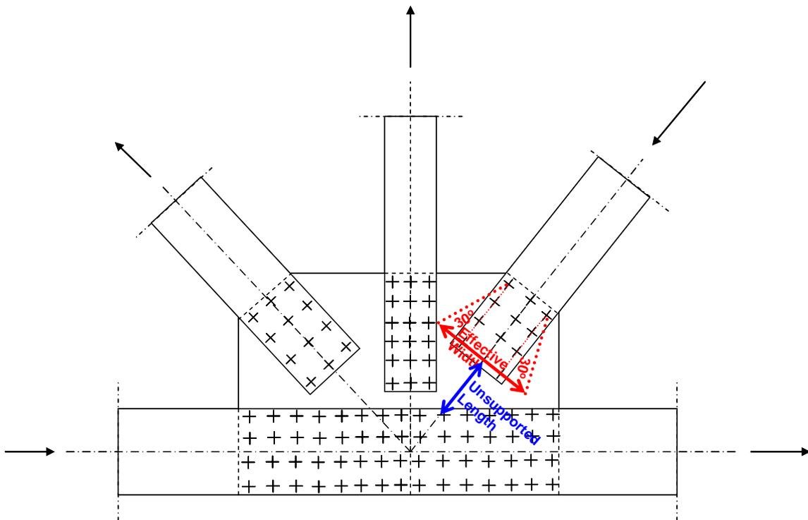
**Figure 6 – Example demonstrating the unsupported length and the use of the Whitmore method to determine the effective width for a gusset plate in compression**
