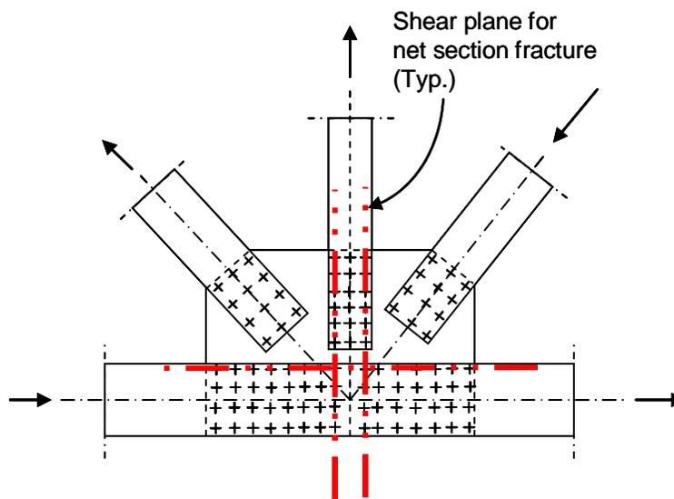
Figure 5 – Examples of net section shear fracture planes
