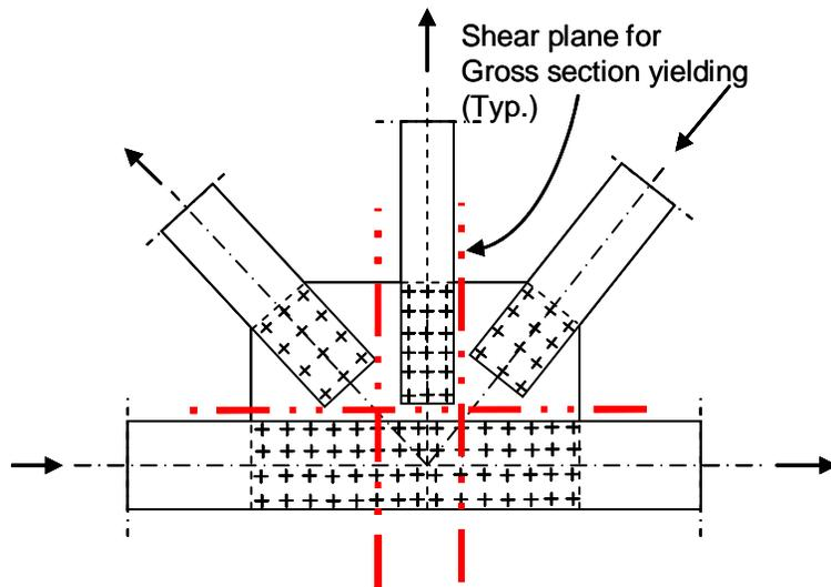
Figure 4 – Examples of gross section shear yielding planes
