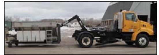
Refurbished 2001 L line with Hook-lift System
