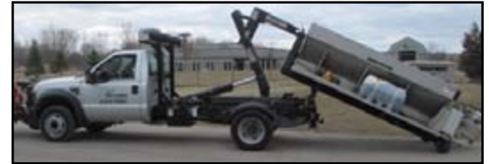
2008 Ford F550 with new Hook-lift System
